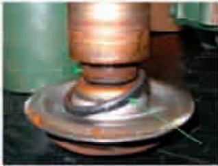
Swollen flange and thrust box O-ring
