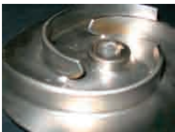
Rotor for FEKA VX 1000 with blades worn by the sand
