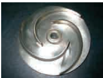
Rotor for FEKA VX 1000 which has worked with sand for 3500 hours (146 days continuous functioning)
