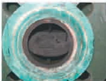
Clapet type valve jammed in mid position due to swelling
