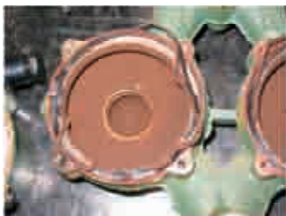
Cause for leak from condensate drain Damaged body seal
