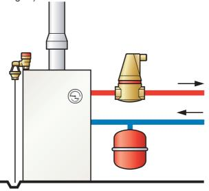
An incorrect, excessive boost pressure may lead to problems. If the system in which a expansion vessel is fitted and an initial pressure of 0.5 bar is filled to 2 bar rather than 0.8 bar. 30% more of the gross capacity will already have been used up before the central heating water expands due to the increase in temperature!
