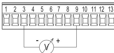
Connection diagram for the external 0-10 V and PWM signals. The 2 signals share the same terminals of the terminal box, and therefore are mutually exclusive.
