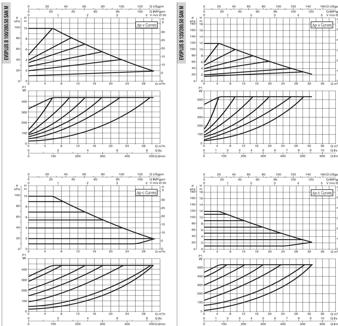
The curves are based on kinematic viscosity values = 1 mm²/s and density equal to 1000 kg/m³. Curve tolerance according to ISO 9906. Fixed speed curves available on the DNA.
