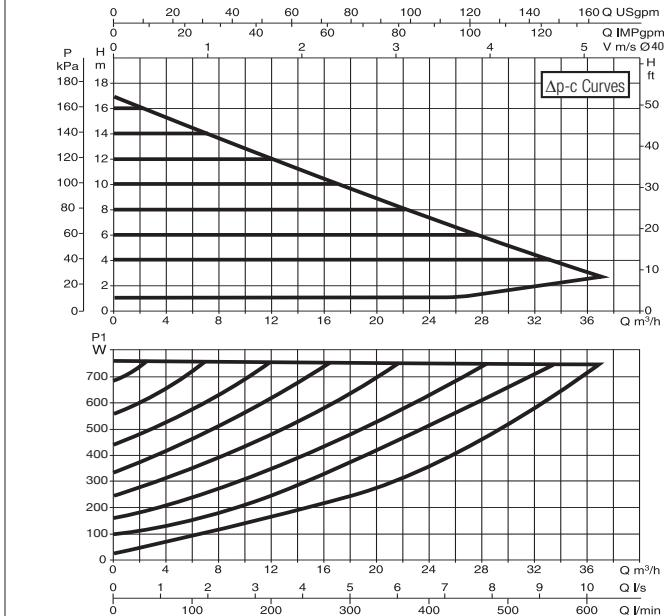
The curves are based on kinematic viscosity values = 1 mm²/s and density equal to 1000 kg/m³. Curve tolerance according to ISO 9906. Fixed speed curves available on the DNA.
