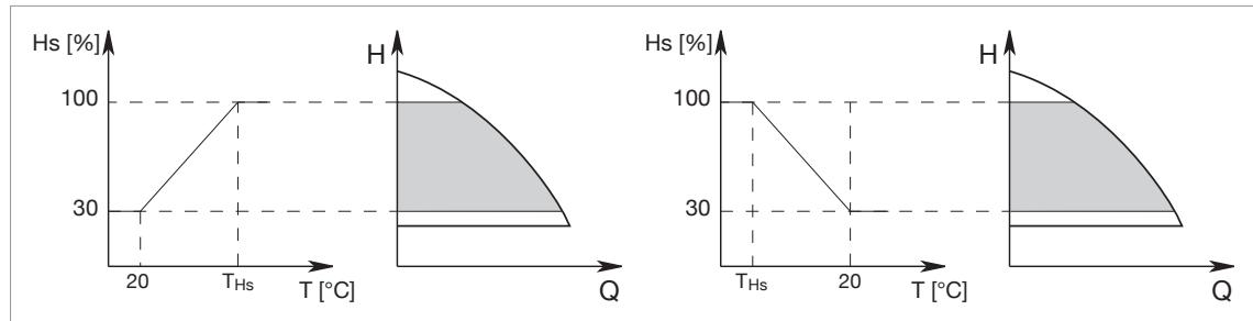
The circulator head set-point is reduced in accordance with the water temperature. The liquid temperature can be set between 0 °C to 100 °C.
