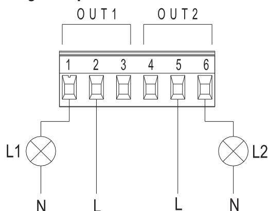
Light L1 comes on when the system includes an alarm, and goes off when no faults are detected, while light L2 comes on when the pump is in operation, and goes off when the pump is stopped.
