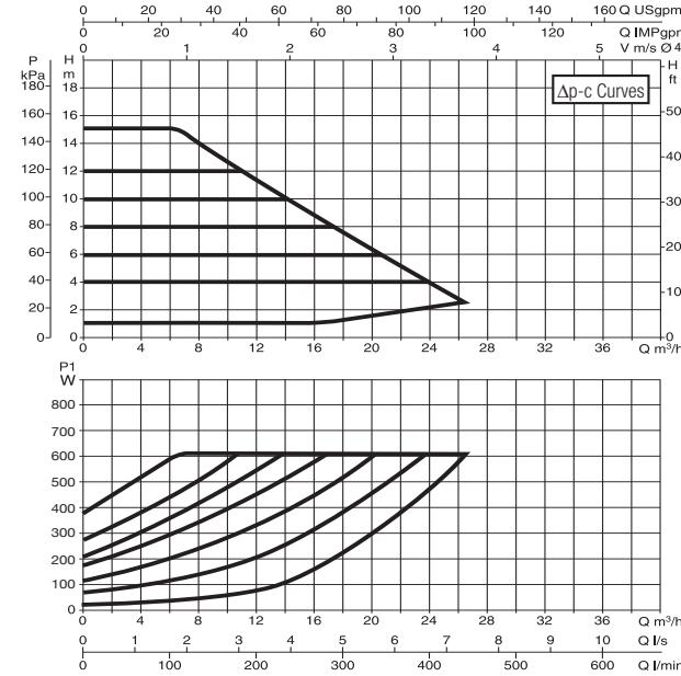
The curves are based on kinematic viscosity values = 1 mm²/s and density equal to 1000 kg/m³. Curve tolerance according to ISO 9906. Fixed speed curves available on the DNA.
