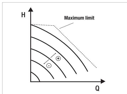
In this control mode, the circulator works based on constant speed characteristic curves. The operation curve is selected by setting the rotation speed using a percentage factor. The 100 % value indicates the maximum limit curve. The actual rotation speed may be affected by the power and differential pressure limitations of the actual circulator model. The rotation speed may be set using the display, or either a 0-10 V or PWM external signal.
