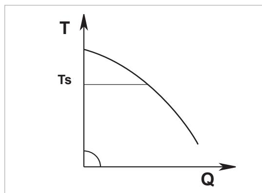
The  $\Delta T_c$  control mode keeps the pumped liquid at constant temperature, changing the flow rate to the  $T_{setp}$  settable value.
