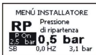
Figure 14: Setting the restart pressure
