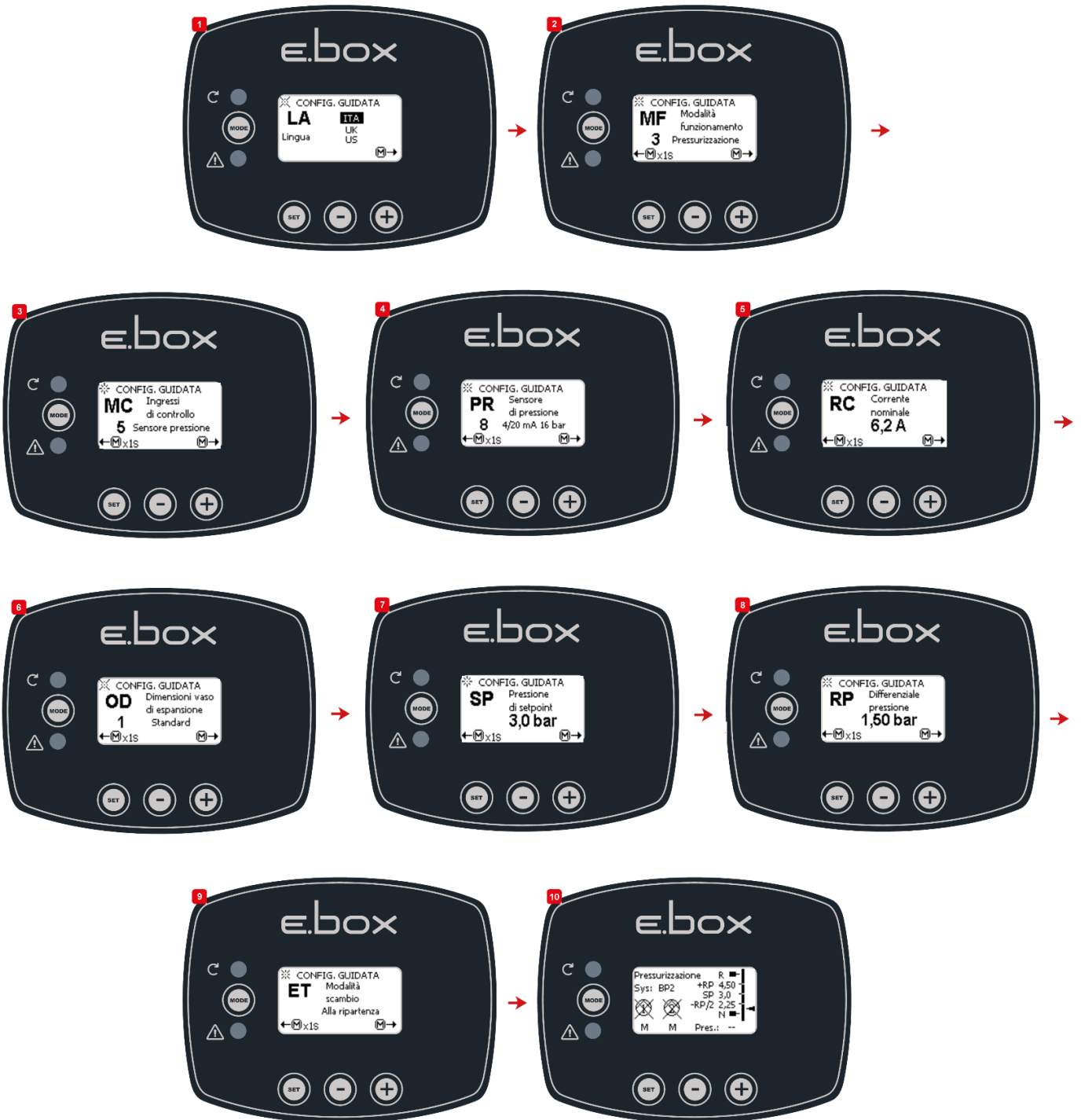
Figure 12: Configuration with a pressure sensor
