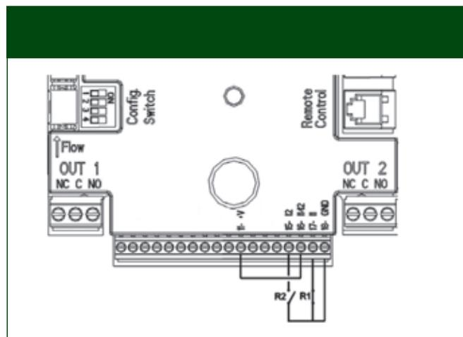
If a voltage is available and not a contact, it can still be used to control the inputs: do not use the +V and GND terminals and connect the voltage source to the input required complying with the characteristics detailed above.
