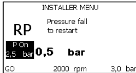
Figure 17: Setting the restart pressure
