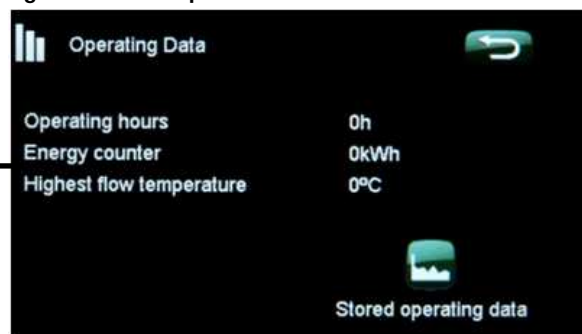
Operating time, energy calculator and highest boiler temperature menu
