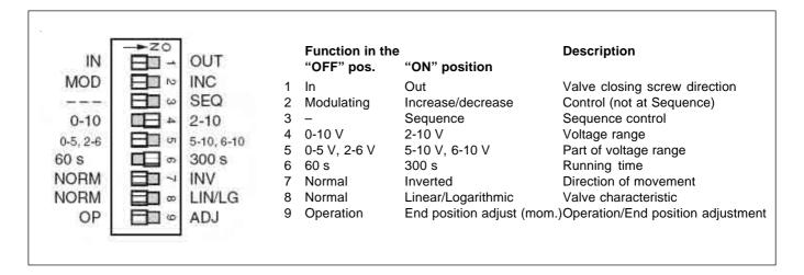
There are nine switches in a row on the circuit board. On delivery ('Factory'), all switches are in the "OFF" position.
