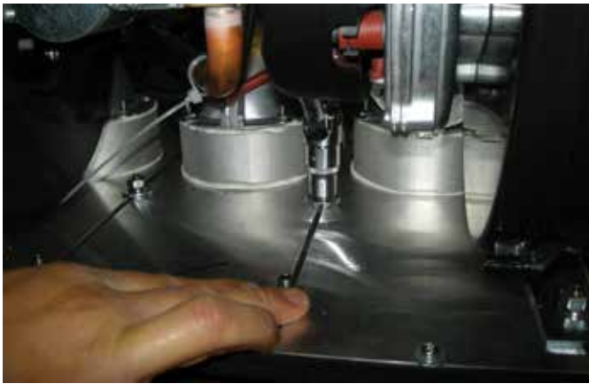
- Remove screws "A" for each element (with 13 mm socket wrench)
