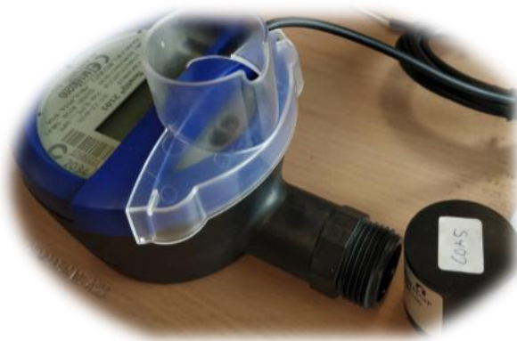
Pulse Interface, type 66-99-143, with Optical Holder type 3026-867 on flowIQ® wired
