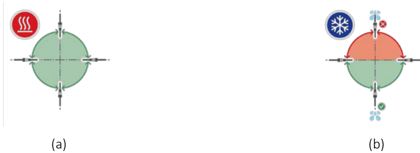
Figure 6. Acceptable orientation of a temperature sensor in (a) a heat and (b) a cooling installation.
