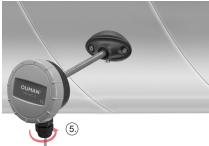
Install the incoming air sensor in central air flow as close as possible to the blower, but far enough in the duct so that air temperature differences are equalized. The exhaust air sensor must be installed on the exhaust air duct in front of the exhaust air fan.
