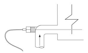
The anticipation sensor measures the temperature of the water from inside the conveyor during consumption. During a time of no consumption the anticipation sensor measures the temperature of circulating water.
