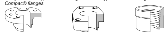
Flanges of DIN Type, Compac® flanges Flanges of SAE Type SAE O-Ring Connections
