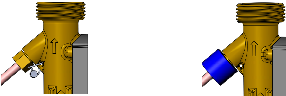
Example of sealing of direct short temperature sensor mounted in a flow sensor
