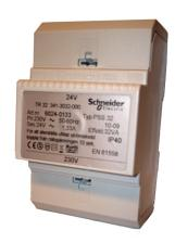
The TR32 and TR60 are transformers moulded in thermoset plastic and mounted in a grey enclosure made of an impact-resistant, self-extinguishing thermoplastic. They can be mounted on a wall or use snap-locking on a 35 mm DIN rail (suitable for modular equipment enclosures).
