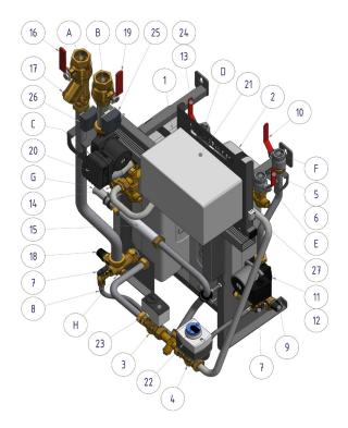
Connections for district heating are welded connections in DN25, for tap water side internal threaded connections in G  $1^{\circ}$  and for heating side internal threaded connections in G11/2".
