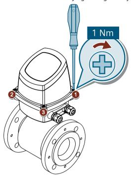
9. To obtain optimum sealing, tighten cable glands.
