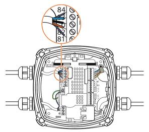
Figure 6-3 Electrode cable with individual wire shields
