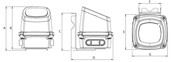
Figure 13-2 Transmitter dimensions wall mounting unit
