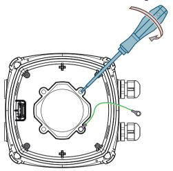
5. Rotate the terminal box and remount it on the pedestal.
