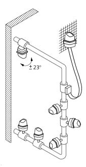
Figure 5-1 Transmitter orientation
