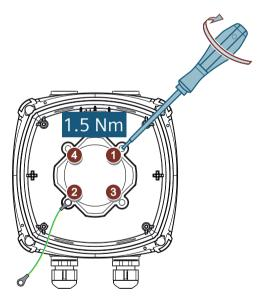
6. Remount the connection board and cables as described in Connecting the transmitter in compact design (Page 40).
