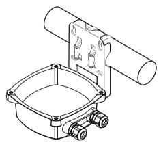
Figure 5-5 Pipe mounting - horizontal
