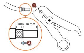
3. Mount cable clamp and remove inner insulation. Remove 7 mm of insulation for each wire.
