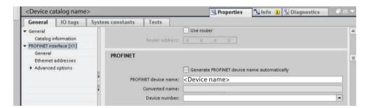
Ensure that the device name matches the device name set in your PROFINET I/O controller or the device will not establish communication with the I/O controller.
