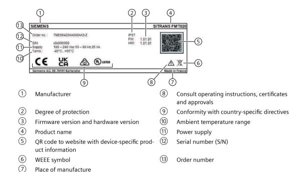
Figure 4-1 Nameplate layout, example
