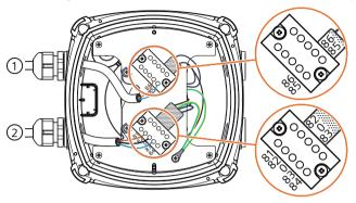
6. Connect the coil and electrode cable shields and grounding cables to the terminal board by using grounding lugs.
