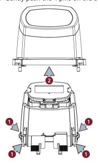
4. Lift off the display and rotate to your desired orientation.
