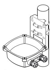
Figure 5-4 Pipe mounting - vertical
