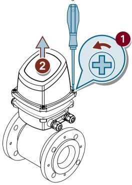
3. Gently push the 4 pins on the bottom side of the transmitter. Lift off the outer case.
