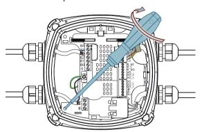
8. Mount transmitter on terminal box by cross tightening as indicated. To avoid damage to the device, do not fully tighten right away .
