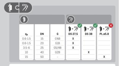
Temperature sensor and flow sensor compatibility. The size of the flow sensor determines which temperature sensors you can use and how to mount them.
