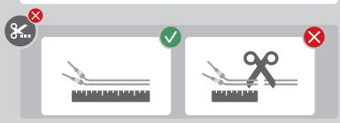
Shortening of temperature sensor cables. It is not allowed to shorten the cables of the temperature sensor.
